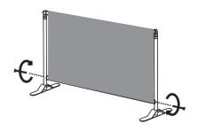
Loosen the telescoping clamps on the vertical poles, adjust the banner to be well displayed,
